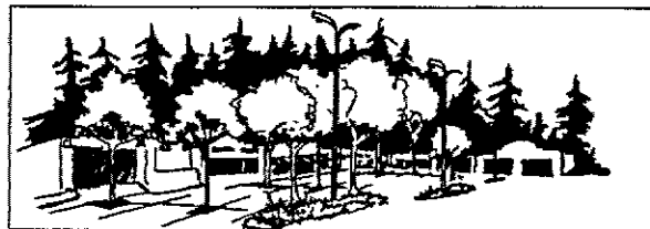
The existing strip mall parking lot retrofit with new landscape installation of one tree for every four parking spaces.
